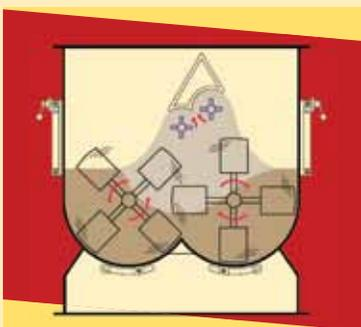
PMS (Pin Mil System) is used when we need to break lumps in the mixture or need higher shear forces during mixing. This system consists of two high speed rotating shafts with welded pins mounted above the fluidized zone.
