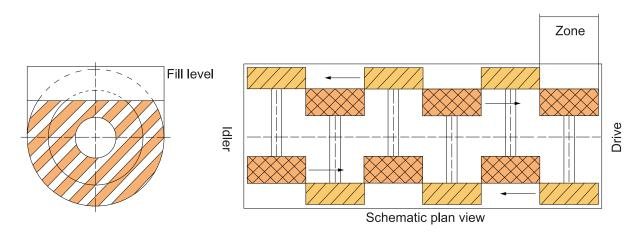
The unique rotor and paddle design divides the housing into smaller zones each served by at least two paddles. All particles are moving hence there is a dynamic transaction between zones, voids are created mechanically and particles are directed to randomly fill the voids. The accuracy and the speed of mixing is achieved by the high volume of voids created for mixing.
