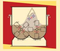
PMS (Pin Mil System) is used when we need to break lumps in the mixture or need higher shear forces during mixing. This system consists of two high speed rotating shafts with welded pins mounted above the fluidized zone.
